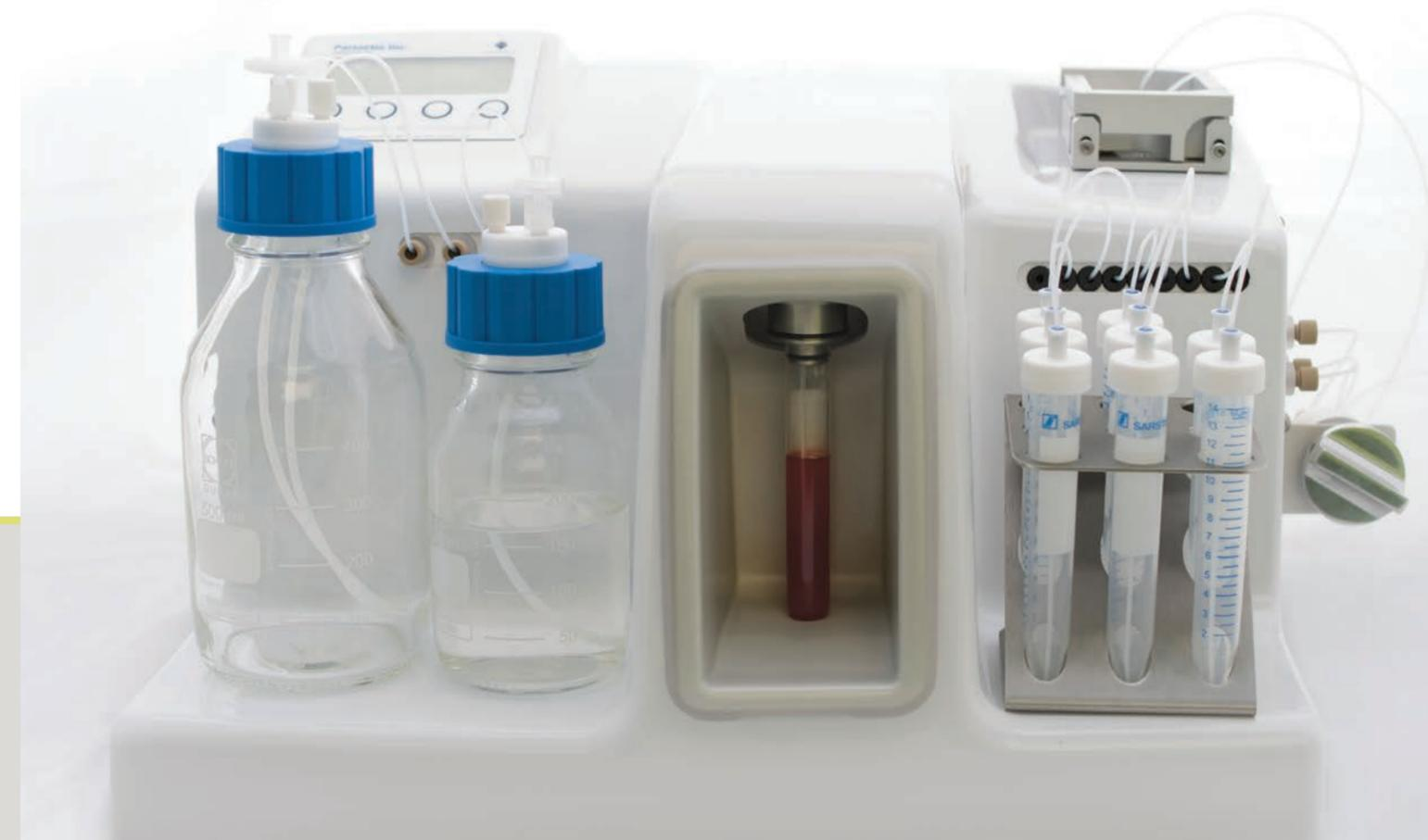
A semi-automated, walkaway system, Parsortix requires no sample pre-processing. Just prime the cassette, insert blood sample test tube, press start and go. Examine cells under a microscope in the cassette, or reverse the flow to harvest cells from the cassette to a test tube for further analysis.
