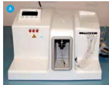
Figure 2. Overview and isolation principle of Parsortix.
