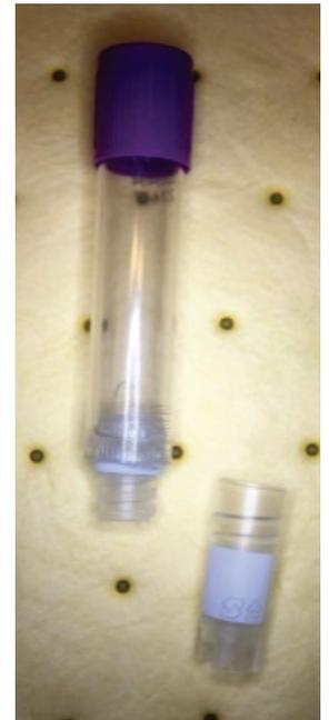
**Figure 1: Prototype of Small Volume Blood Adaptor**
