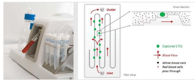
Fig. 1 – Parsortix™ instrument and the mechanism of separation.
