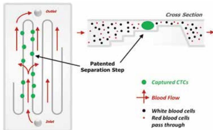
CTCs are caught on a 10µm-step that criss-crosses the microscope slide sized disposable cassette. Blood cells pass through and are washed away by rinsing the cassette with buffer.
