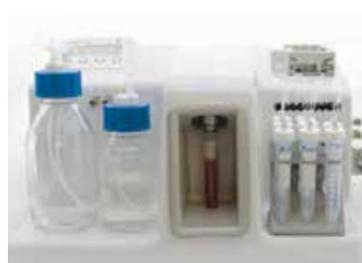
The Parsortix system from ANGLE uses a patented micro-fluidic technology to isolate rare cells (e.g. CTCs) based on their less deformable nature and larger size compared to other blood components.
