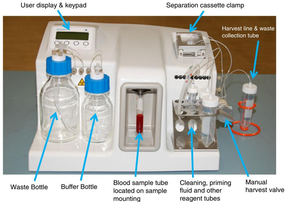
**Figure 1.** Parsortix™ PR1 Cell Separation System.
